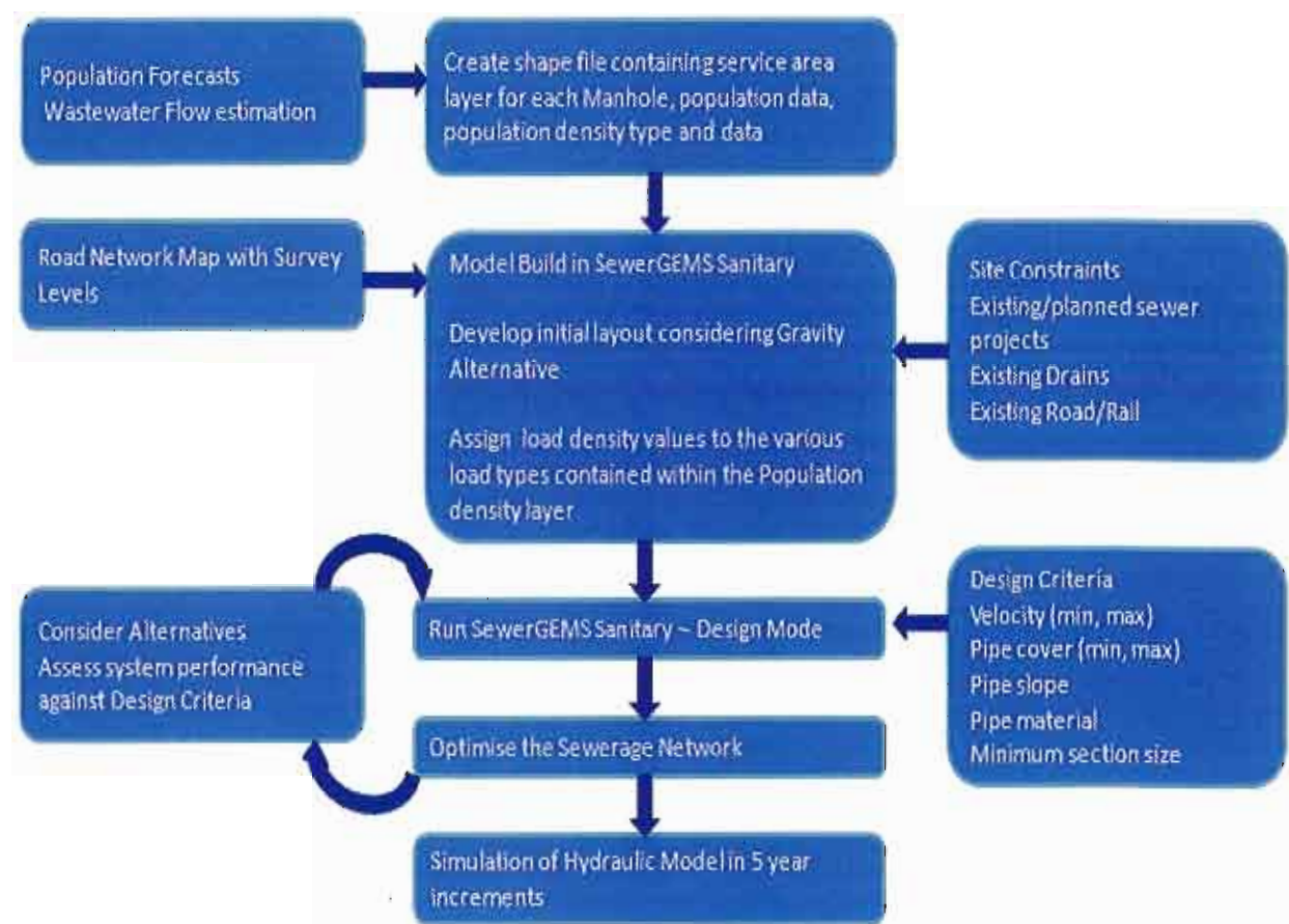
Figure 7.4: Procedural Flow Chart of Sanitary SewerGEMS
