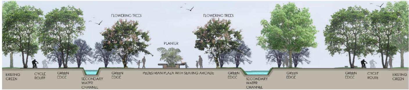
Proposed section of secondary channels to Najafgarh Waterway
