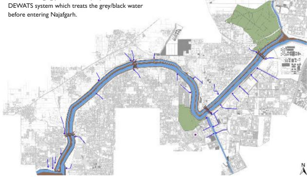
Map showing existing natural drainage drop points and flow lines to the Najafgarh Waterway
