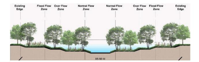
Section showing the proposed edges in steps of the waterway by cut and fill method
