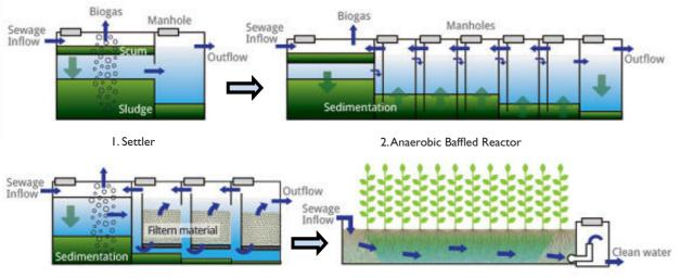
3. Anaerobic Filter
